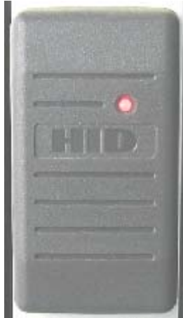
Figure 2-15 Bi-color LED in a Security Device
